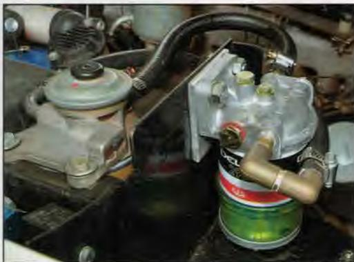
to bypass, we drilled a hole through the filter, allowing fuel to pass. It worked. Back home and wanting a permanent fix, I decided on a quality second fuel filter system with a water catchment bowl. But there wasn't room in the engine bay for a match with the wood scraped off let alone a filter assembly.
